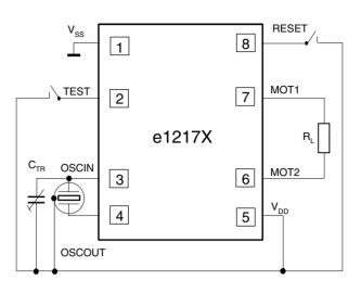
Range of trimmer capacitance:  $C_{TR} = 5 \text{ pF}$  to 30 pF
